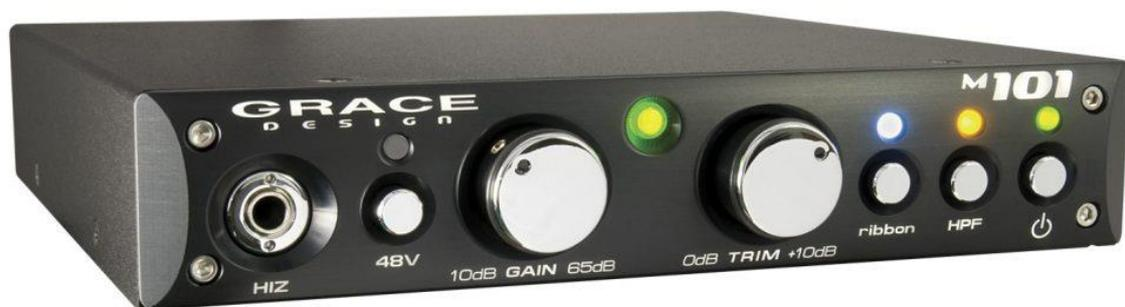
The preamp is an amplifier used to amplify the electrical signals generated by the mic and converts them into a language that your computer or recording software can understand.
